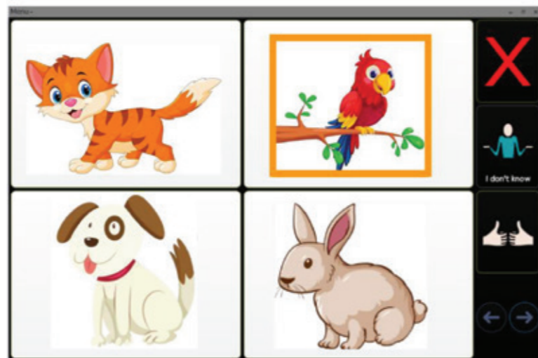
Here is an example of a test question. The child is asked to 'find bird' and the computer scans through the different pictures and when the orange box is around the bird, the child makes their selection with the switch.
