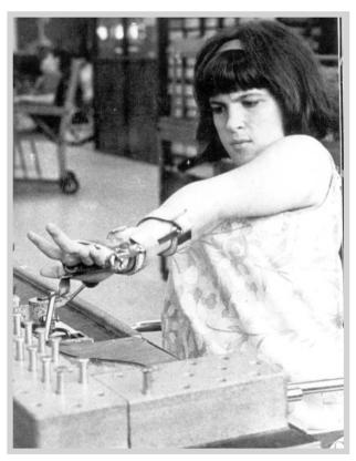
Carmella Kirkman assembling a core and cheek in an automatic press. Note that the hand splint provides a fork for the component part.
