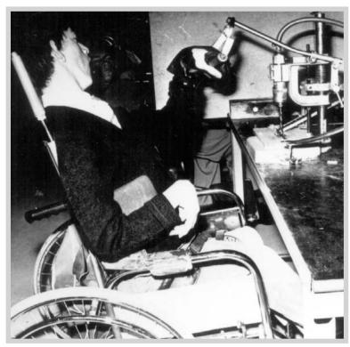
Brian Freestone operates a drilling machine that has been adapted to an automatic operation of feed and displacement.
