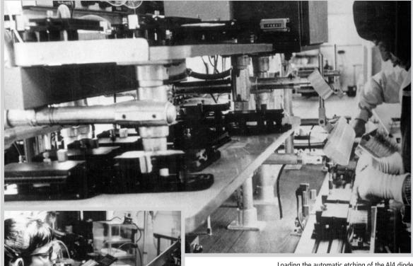
Loading the automatic etching of the Al4 diode.
