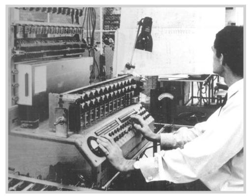
L.M.E. combination test unit applicable to L.M.E. Xbar sets or 2,000 switching sets.
